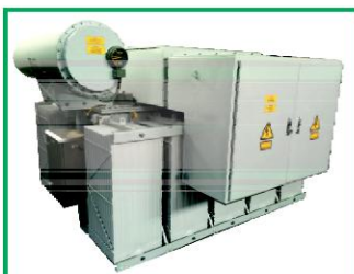
5070 kVA, 10000/4x1903 V, 24 Pulse Converter Transformers for petro-chemical industry
